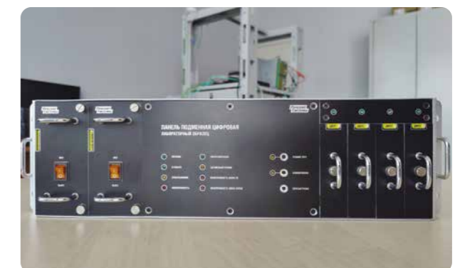
External view of the RPA panel with the substitution function.
